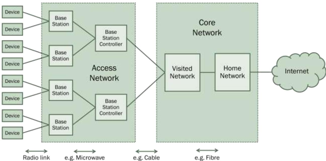
**Figure 1 - Cellular Network Architecture with Intermediate Communications Links**
